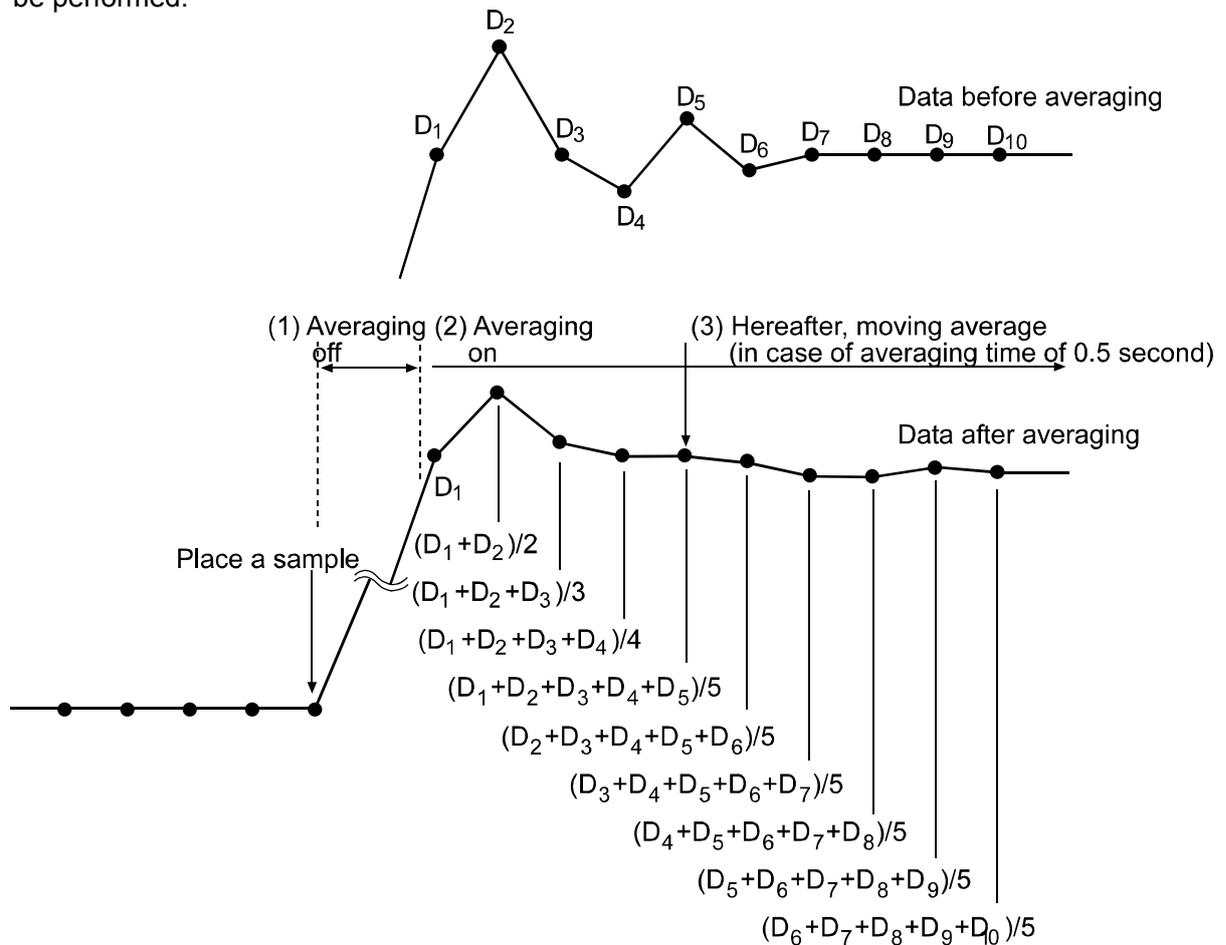
When a small amount of sample is weighed or is filled, the fluctuation of a weight value is too small to be beyond the selected range and the averaging operation is not disabled. Consequently moving averaging is always performed and it takes a longer time to reach the final weight value. Under such a situation, change the setting of " $F I-b$ " to a smaller range. But please note that the smaller the range is, the more prone to external disturbance the value will become.
